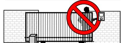
DO NOT mount operating devices accessible through the gate or in between gate and wall.
